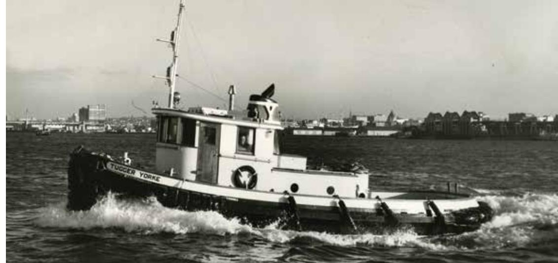
showing little in common with the original other than the hull) was designed in April 1950, and built by Victoria Machinery Depot for Black Ball Towing Co. Ltd. Dimensions were 42.7’ x 15.1’ x 6.3’. A highly innovative feature was a hydraulically elevating wheelhouse, indicating that the tug needed to duck some bridges! At some point it was extensively rebuilt. It was still registered in 2003 and owned by a numbered company in Kitimat, but the registry of the tug closed in 2011.
