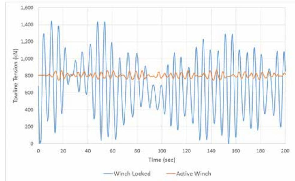
Figure 1: Towline Tension during an Escort Manoeuvre in Waves
