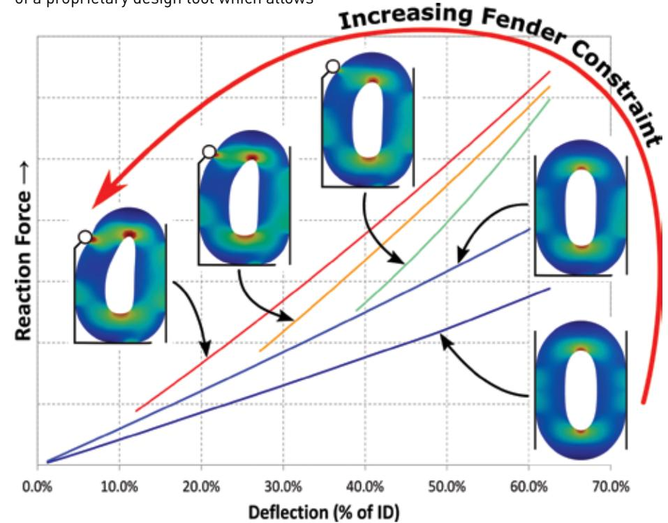
Impact of increasing levels of constraint on fender stiffness.
