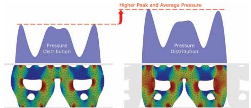
Comparison of the pressure distribution and deformed shape of an isolated w-fender (left) with an array of closely packed w-fenders (right).
