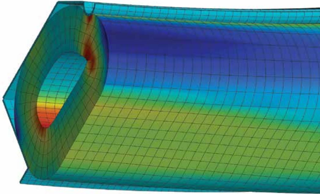
Example of a 3D non-linear finite element analysis for a cylindrical fender on a curved bow section.
