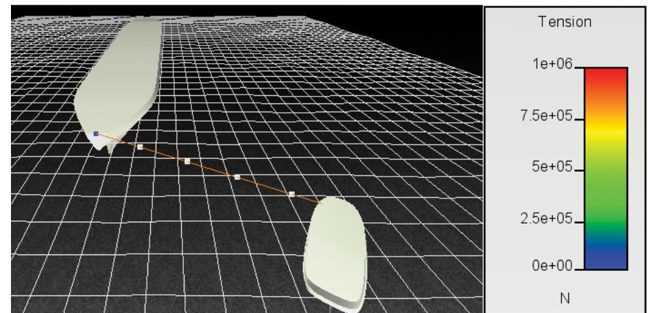
Figure 2: Simulation of a RAStar Escort Tug Applying Steering Force to a Tanker
