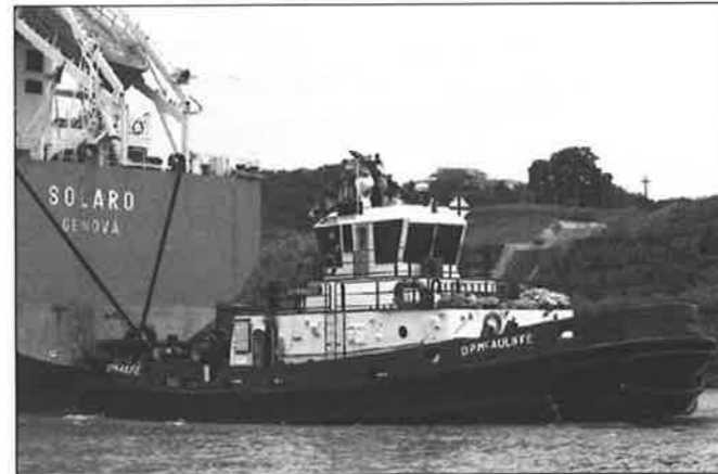
Figure 7: Typical tug-ship bridle connection configuration used in Panama Canal. Photo courtesy of Capt Max Newman, Panama Canal Authority.
