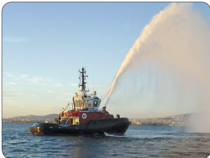
Seaspan Raven — Fi-Fi 1 capability — 2400m 3 /hr pumping capacity.
