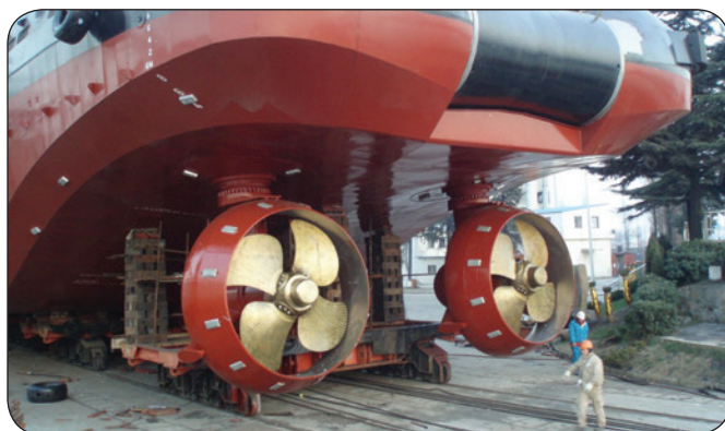
Z-drive units in the stern of an ASD tug.
