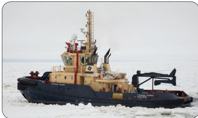
Svitzer Aniva — one of four TundRA 3400 Class icebreaking escort tugs for support of the LNG terminal at Sakhalin, Russia.
