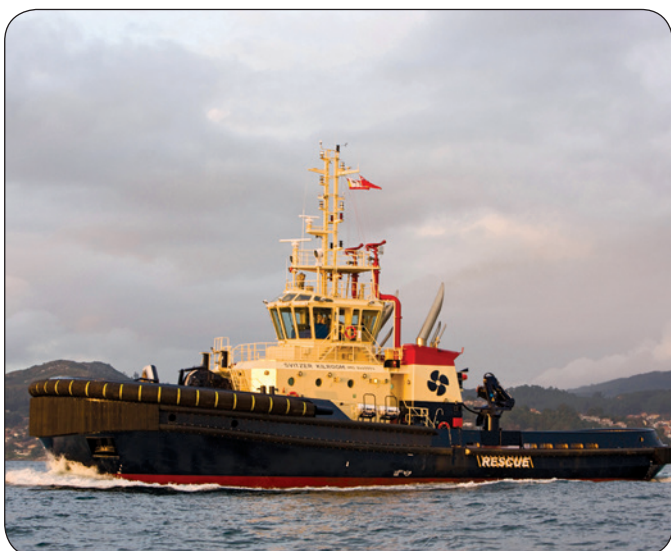
Svitzer Kilroom — 39 metres, 116 tonnes bollard pull.
