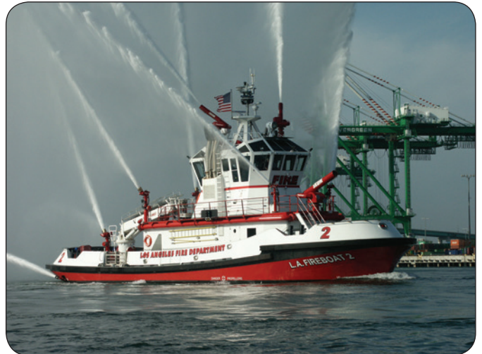
Warner L. Lawrence — a VSP powered fireboat.
