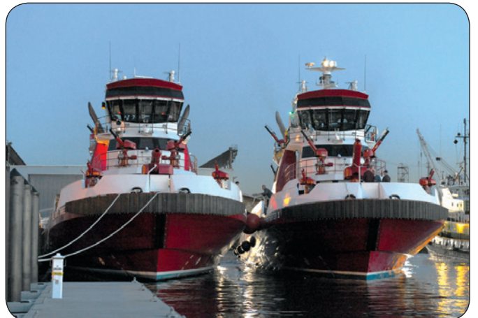
Firefighter 2 and Three Forty-Three — two 42-metre, 11,500 cu.m/hr, 18-knot fireboats for FDNY.
