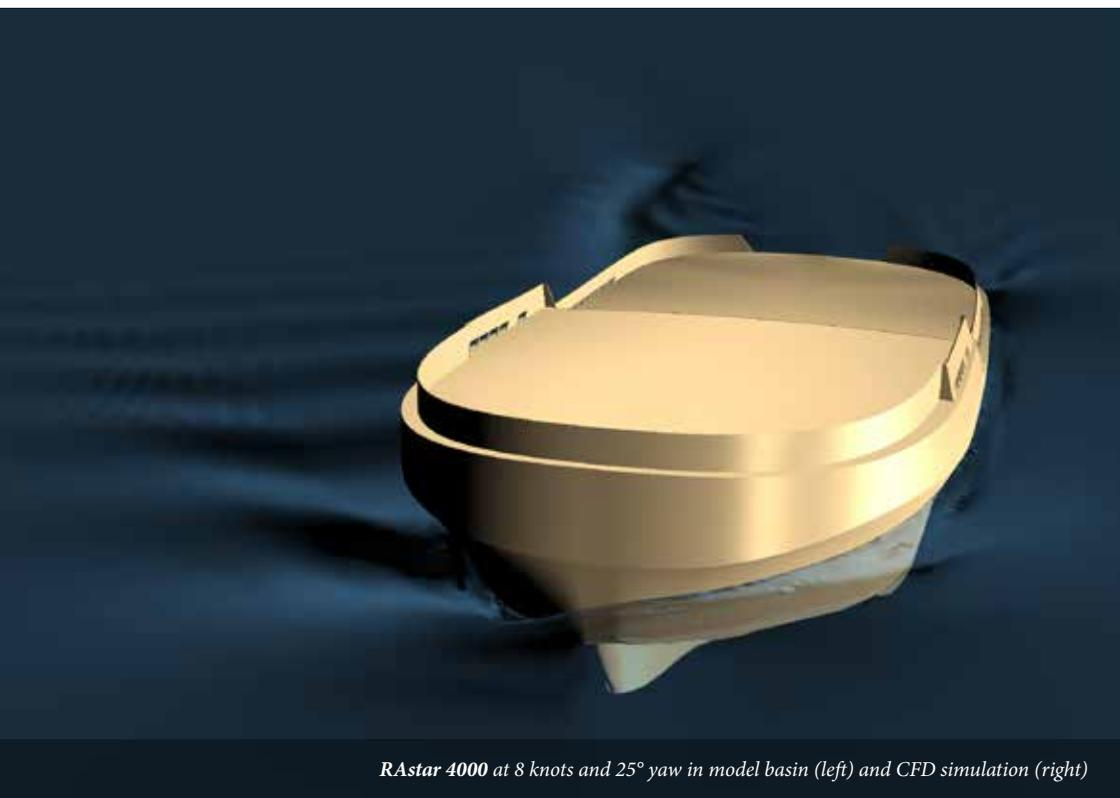
*RAstar 4000 at 8 knots and 25° yaw in model basin (left) and CFD simulation (right)*
