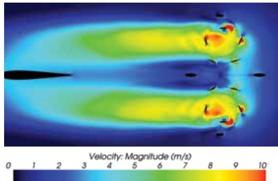
Figure 2: Plan view of velocity contours at mid-height of VSP blades
