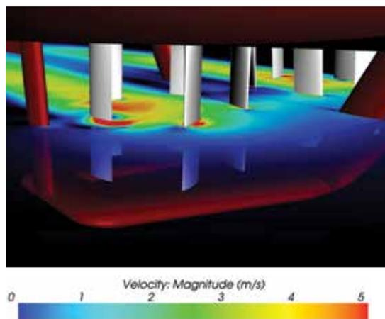
Figure 3: Perspective view of velocity contours at mid-height of VSP blades
