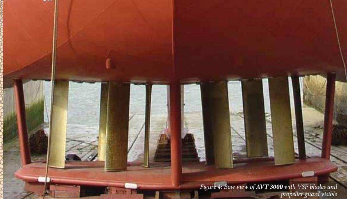
Figure 4: Bow view of AVT 3000 with VSP blades and propeller guard visible
