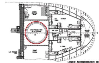
LNG tank hold location and storage capacity is challenging for small vessels: e.g. a 90t tug
