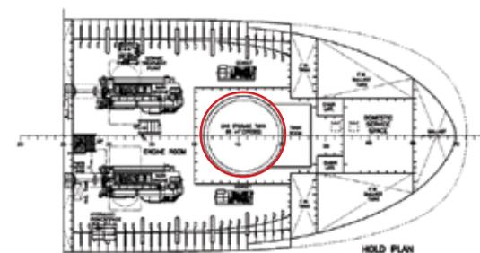
80 m<sup>3</sup> gross equals about 70 m<sup>3</sup> useable, about 35 hrs at full load and about 110 hrs at average loads
