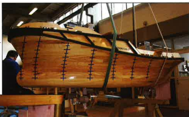
The 1/12th scale model of the Escort Rotor Tug for the tank tests (photo above). The inset photo shows the model's aft end with Z-drive, skeg and flap (which was eliminated after model tests). Main characteristics of the full-
