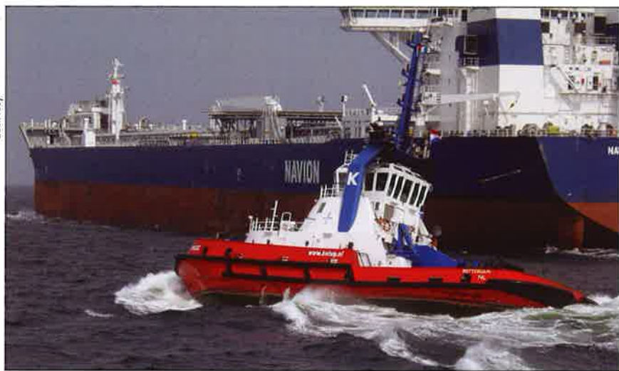
The Rotor tug RT MAGIC in the escort mode, running bow first.
