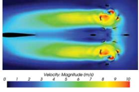
Figure 2: Plan view of velocity contours at mid-height of VSP blades
