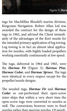
Cedar so out-performed their open-screw sister ships that within a very short time the open-screw tugs were converted to nozzles as well. The conversions however were to fixed nozzles rather than steering nozzles. Of significant interest is how the speed of the nozzle tugs was also substantially higher, as well as the 25% increase in BP values.
